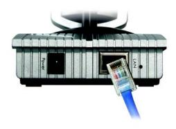
Figure 4-1: Connect the Ethernet Network Cable
